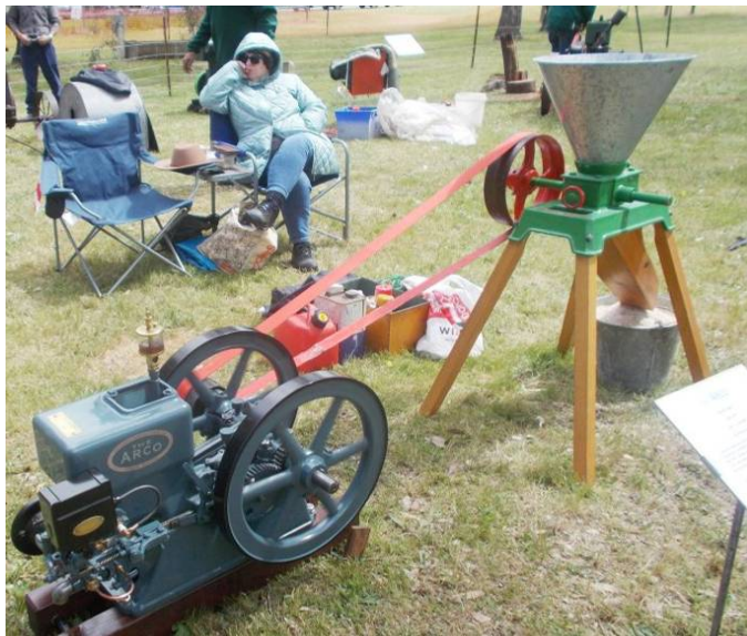
← A unusual 1924 American Arco engine driving a grain grinder . Owner David Hawkins all the way from Batlow NSW
