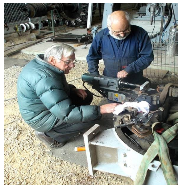
Phil and Hayden using a magnetic drill to enlarge a mounting hole on the large Willans Diesel at the Steam Club. He could turn his hand to anything!
