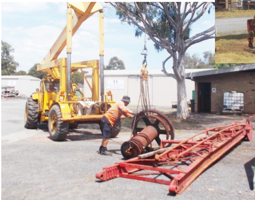
Undercarriage and machinery deck of the rail mounted steam crane. Very deteriorated and dismantled yet an interesting exhibit once assembled. We have the vertical cross tube boiler which mounts on rear counterweight (just in front of the dog man). It is a heavy little lump, what you see is just under 20 tonnes
