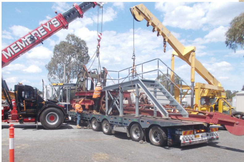
Undercarriage and machinery deck of the rail mounted steam crane. Very deteriorated and dismantled yet an interesting exhibit once assembled. We have the vertical cross tube boiler which mounts on rear counterweight (just in front of the dog man). It is a heavy little lump, what you see is just under 20 tonnes
