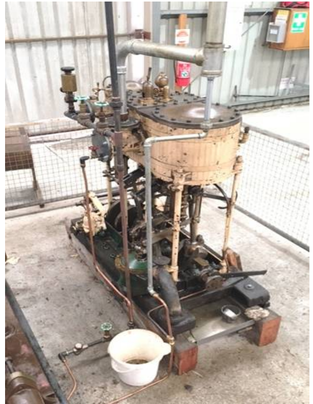
The engine is the first one you see when you come in the main door of Bay 1 . It is a fairly small 2 cylinder doube acting compound engine with heavily counterweighted crank shaft but very light rod frame between the bedplate and cylinder block . Obviously made for power and light weight not long life. Warwick pic
